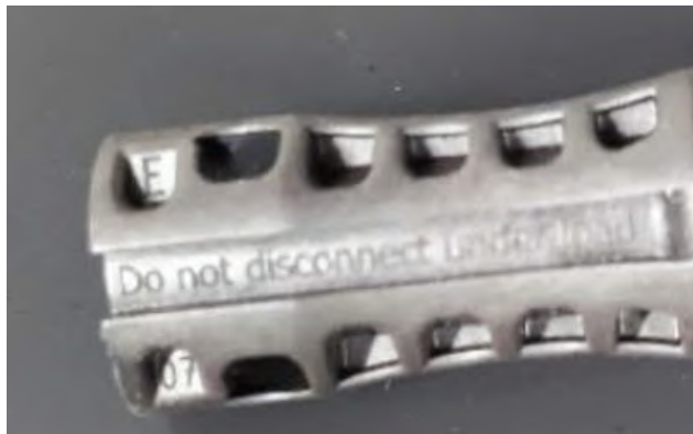
Mark (Do not disconnect under load)
