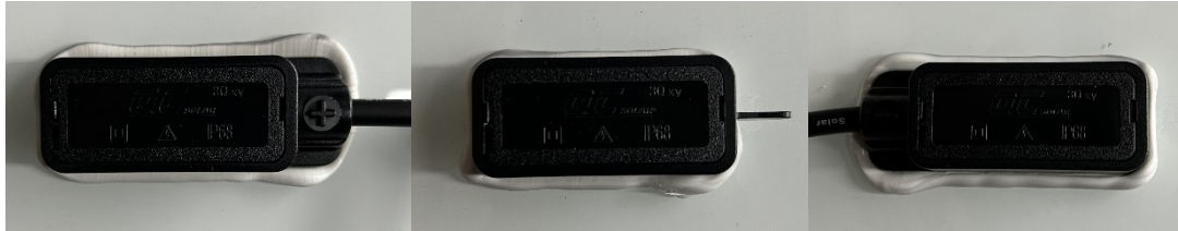
Fig. 7: View of junction box of module type SR-54M435NHLProD
